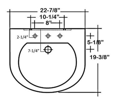
Dimensions of fixture are nominal and may vary within the range of tolerances established by ASME Standard A112.19.2-2013. Dimensions and specifications subject to change without notice.
